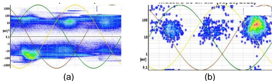
Figure 1. Example of PD signals before (a) and after filtering: external surface discharge (b).
