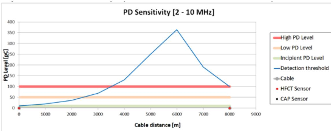
Figure 5. Analysis of sensor sensibility vs distance for a concrete circuit.
