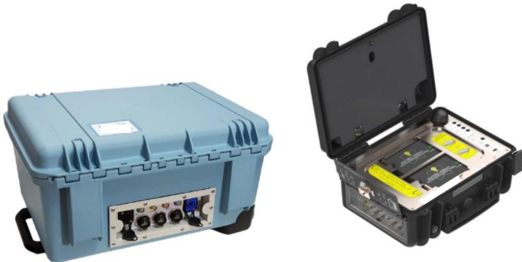
*Figure 3. Portable PD measure equipments*
